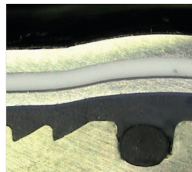
O-ring na persing TH-profiel
